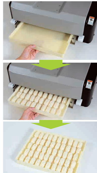
Automatic alignment starts when tray is set
